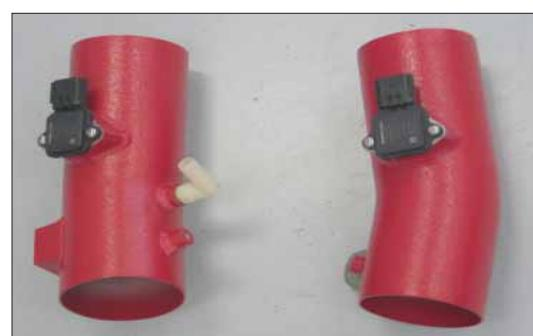
16. Install the mass air sensors into the K&N® intake tubes and secure with the provided hardware.
