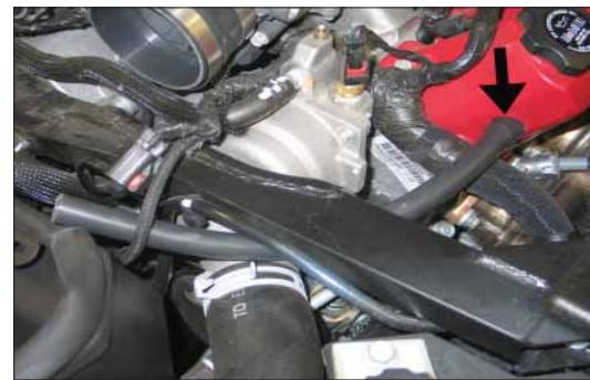
13. Install the provided crank case vent hose onto the valve cover port as shown and secure with the provided tie wrap.
