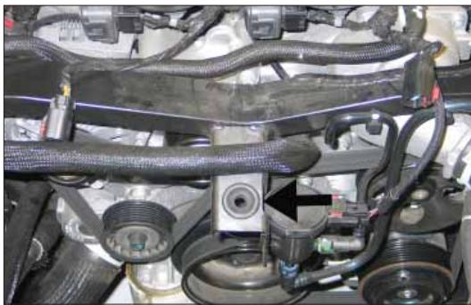
7. Remove the rubber mounting grommet shown.
