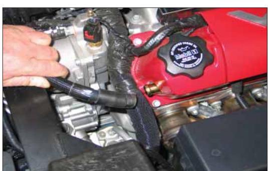
5. Cut the tie wrap which secures the vent hose to the valve cover port. Then unhook the crank case vent hose as shown.
