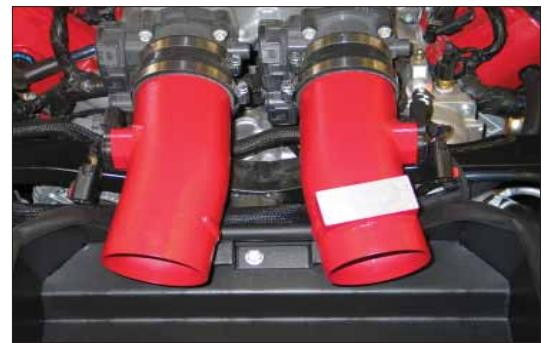
19. Align the intake tubes so that they are straight and even coming out of the throttle bodies, then tighten the heat shield mounting bolts and tube mounting bolts.
