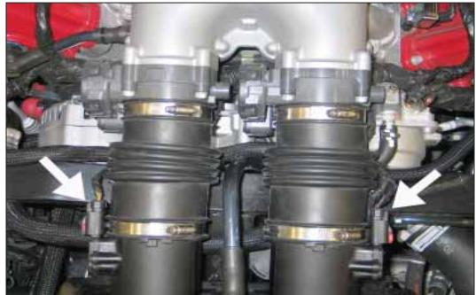
2. Release the locking tabs and then disconnect the two mass air sensor electrical connections.
