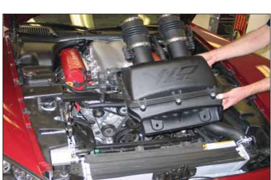
6. Dislodge the air box assembly from the mounting grommet and remove the air box from the vehicle.
