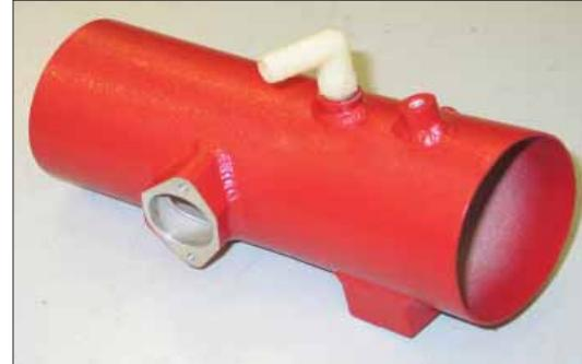
14. Install the 90° vent fitting into the left side K&N® intake tube as shown.
