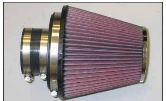
21. Install the silicone hoses (084052) onto the filter adapters and secure with the provided hose clamps.
