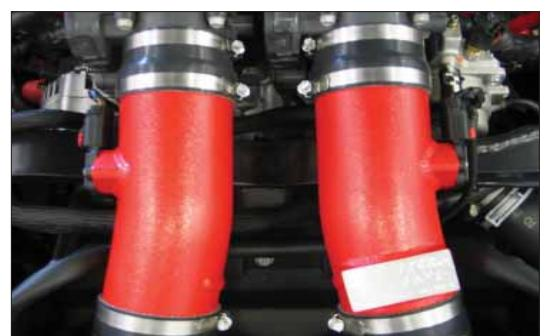
23. Reconnect the mass air sensor electrical connections.
