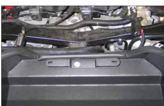
11. Install the tube mounting bracket (083109) into the heat shield and secure with the provided hardware.
