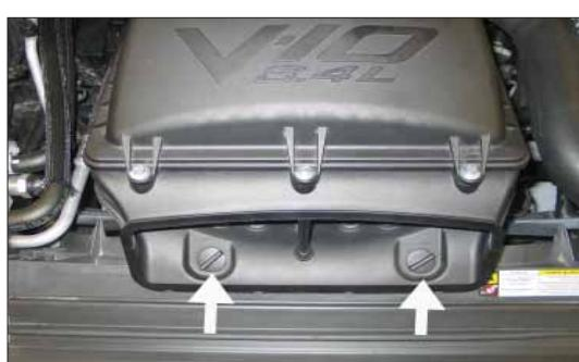
4. Unscrew and remove the two air box fastener nuts shown.
