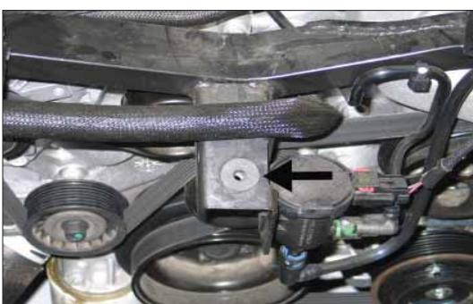
9. Install the provided nut insert into the air box mounting grommet hole as shown.
